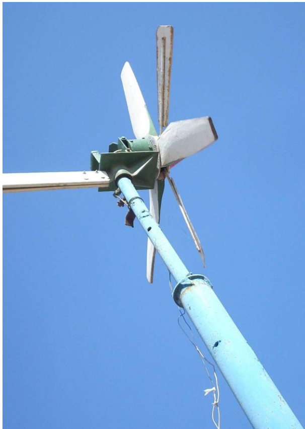
Figure 1. "Old model" small wind turbine installed to provide electric power to the community building at Hanchon Ward.
