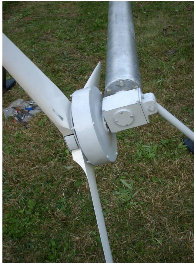
Figure 4. Top section of the new model 300-W SWES with the axial-flux permanent-magnet disc generator before installation at the UNDP premises.
