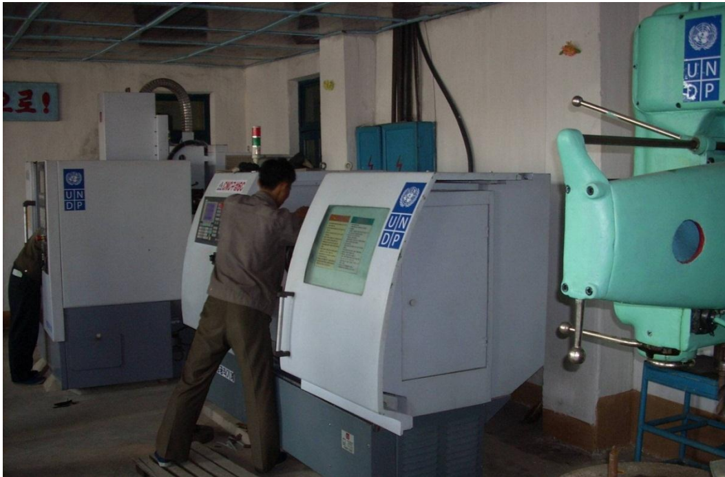
Vertical drill machine, CNC lathe and CNC drill machine installed at the SAOS/CWERD manufacturing workshop.
