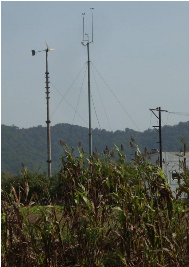
Figure 3. The new 300 W turbine at the CWERD test field with the MEASNET-conform wind mast.
