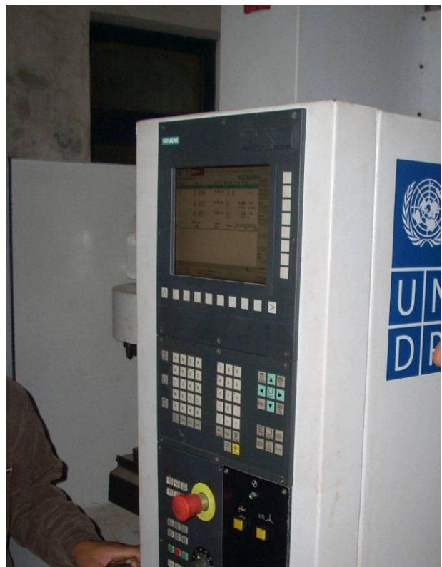
Control panel of the CNC vertical drill machine.
